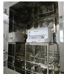
Measurement of substances released by products
