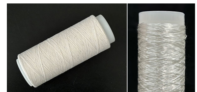
Cotton-recovered cellulose fibers processed with Dry Fiber Technology (left: spinning, right: wet spinning)
