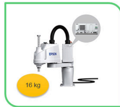
The T3 has a built-in controller
