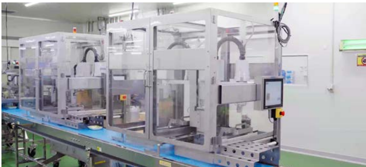
Food packing robot system that employs T3-B robots
