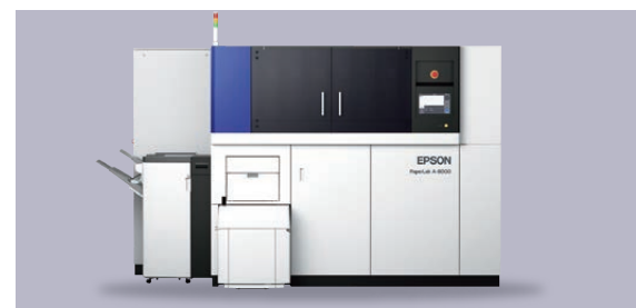
The PaperLab A-8000 office papermaking system produces new paper from used paper (2016)
