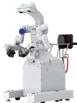
Autonomous dual-arm robots have arms that move independently to perform tasks
