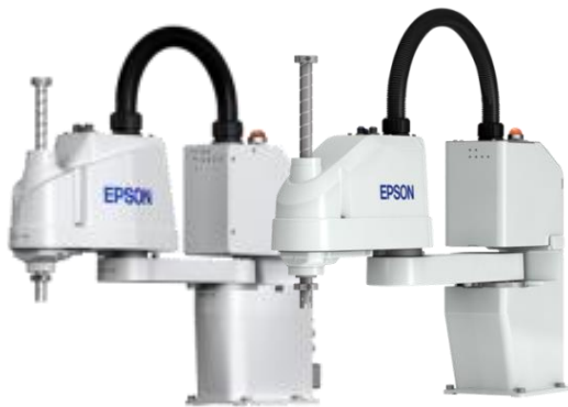
SCARA robots with integrated controllers (T series)
